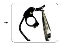
10. Slide the cable into the guide under the lever, cut the cable in appropriate length and fix the cable end.
